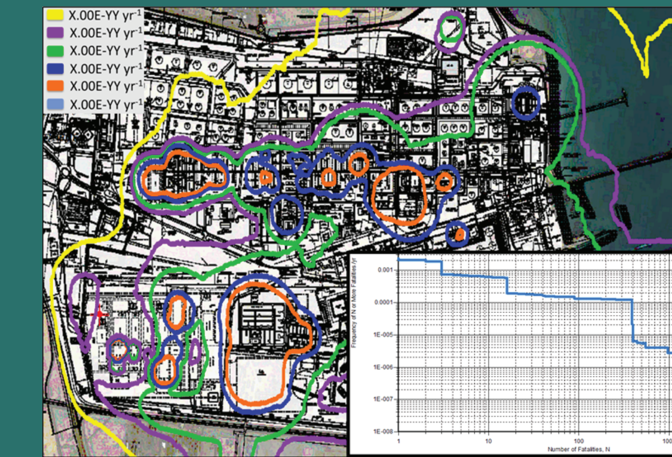
Figure 02 Example of QRA Results: Individual Risk Contours and FN Curve
