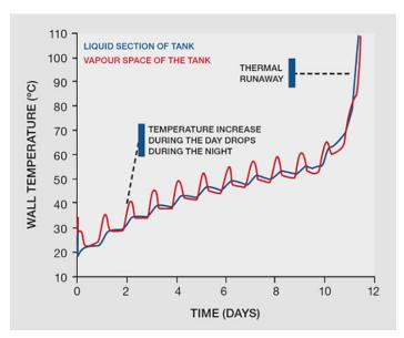
An example of the dynamic modelling of a vessel under solar heating, which results in a thermal runaway reaction.
