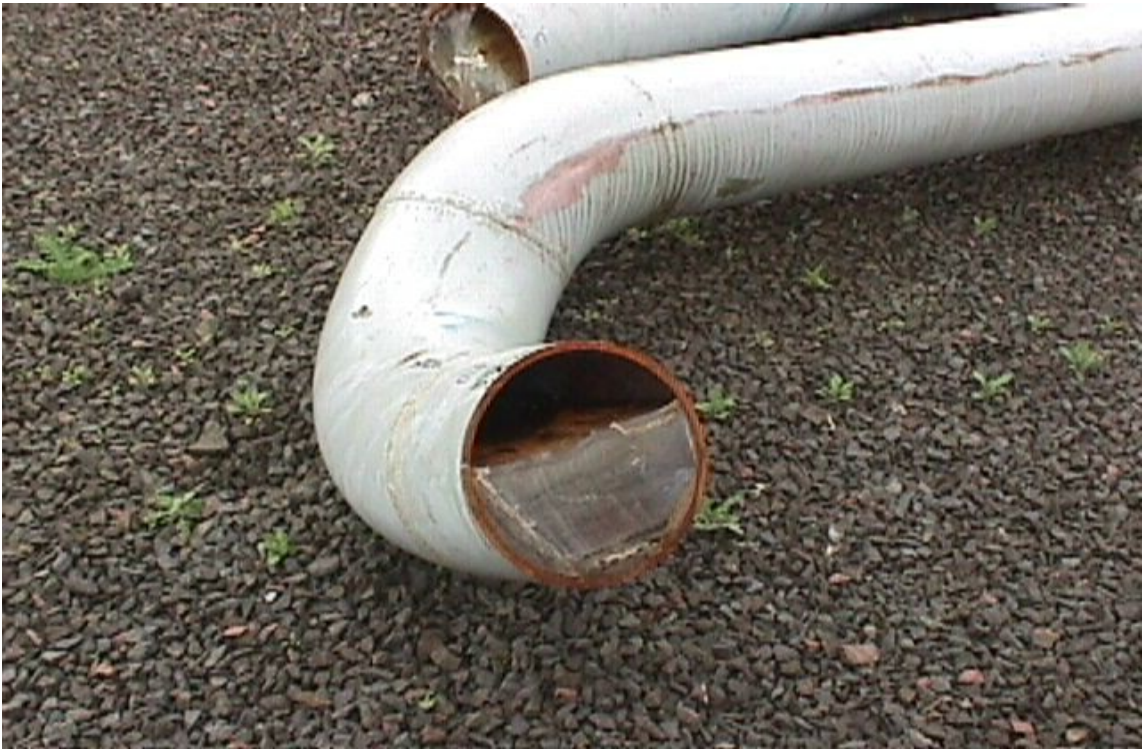
Figure 4 – Reaction Force Example – Failure of Unsupported Piping
