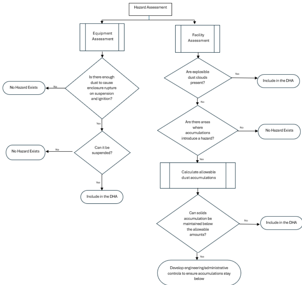
Figure 1: Combustible Dust Hazard Assessment Flow
