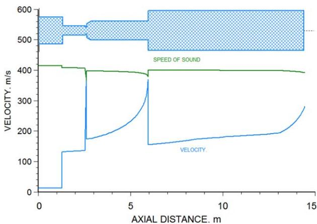
**Figure 10.** Case study C—Pipe segments velocity profiles. [Color figure can be viewed in the online issue, which is available at [wileyonlinelibrary.com](http://wileyonlinelibrary.com).]
