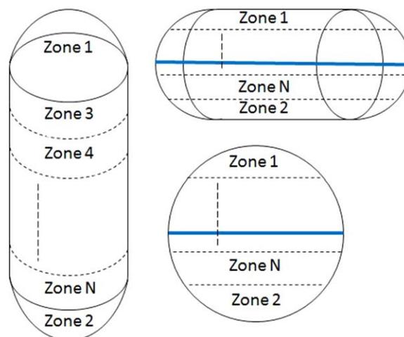
**Figure 13.** SuperChems expert vessel segmentation scheme. [Color figure can be viewed in the online issue, which is available at [wileyonlinelibrary.com](http://wileyonlinelibrary.com).]
