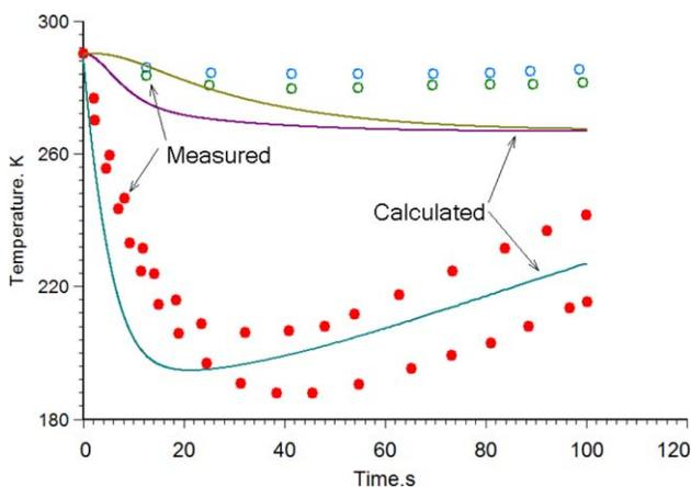
**Figure 8.** Case study B—Fluid and wall temperature predictions. [Color figure can be viewed in the online issue, which is available at [wileyonlinelibrary.com](http://wileyonlinelibrary.com).]
