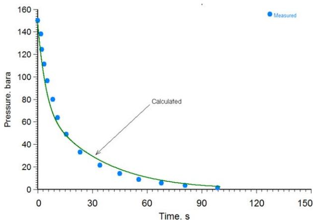
**Figure 7.** Case study B—Calculated pressure profile. [Color figure can be viewed in the online issue, which is available at [wileyonlinelibrary.com](http://wileyonlinelibrary.com).]
