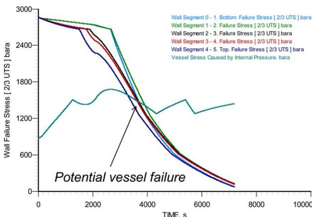
**Figure 5.** Case study A—Predicted failure pressure. [Color figure can be viewed in the online issue, which is available at [wileyonlinelibrary.com](http://wileyonlinelibrary.com).]
