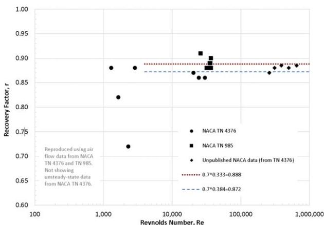
**Figure 12.** Measured values for the wall temperature recovery factor [8]. [Color figure can be viewed in the online issue, which is available at [wileyonlinelibrary.com](http://wileyonlinelibrary.com).]
