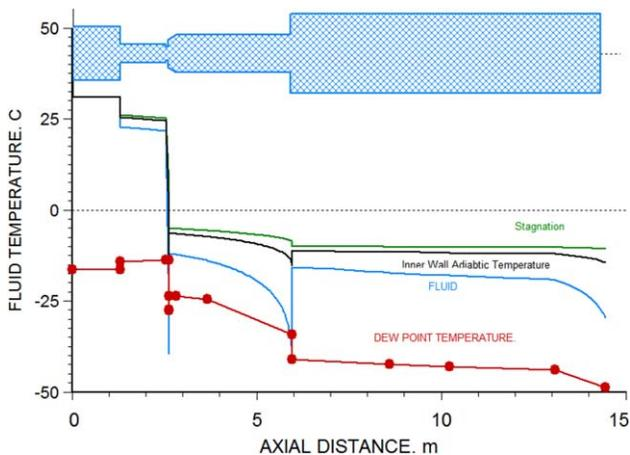
**Figure 11.** Case study C—Piping segments temperature profiles. [Color figure can be viewed in the online issue, which is available at [wileyonlinelibrary.com](http://wileyonlinelibrary.com).]
