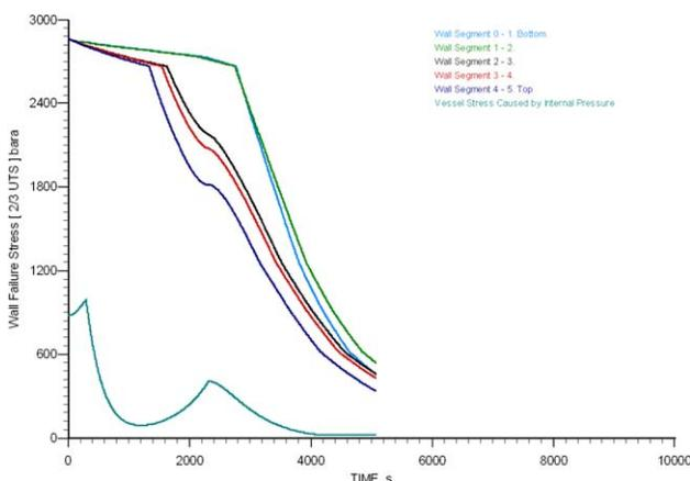
**Figure 6.** Case study A—Predicted failure stress with an emergency depressuring valve. [Color figure can be viewed in the online issue, which is available at [wileyonlinelibrary.com](http://wileyonlinelibrary.com).]
