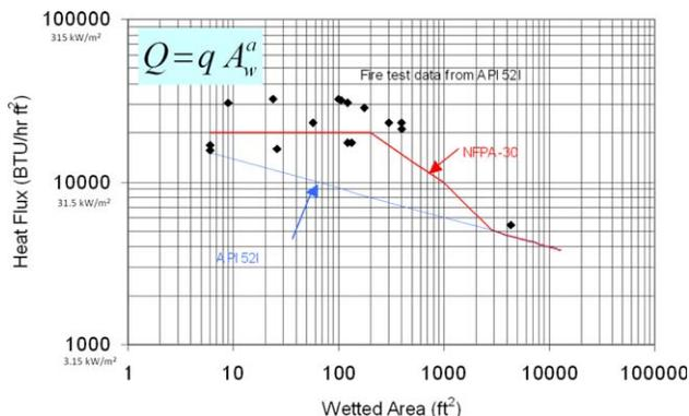
**Figure 1.** NFPA-30 and API-521 fire flux correlations. [Color figure can be viewed in the online issue, which is available at [wileyonlinelibrary.com](http://wileyonlinelibrary.com).]
