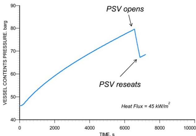
**Figure 3.** Case study A—Vessel pressure history. [Color figure can be viewed in the online issue, which is available at [wileyonlinelibrary.com](http://wileyonlinelibrary.com).]
