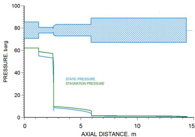
**Figure 9.** Case study C—Pipe segments axial pressure profiles. [Color figure can be viewed in the online issue, which is available at [wileyonlinelibrary.com](http://wileyonlinelibrary.com).]
