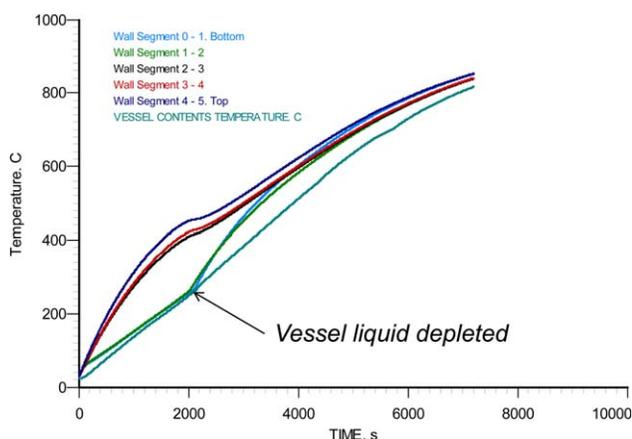
**Figure 4.** Predicted wall segments temperatures using SuperChems Expert<sup>TM</sup> and Eq. 3. [Color figure can be viewed in the online issue, which is available at [wileyonlinelibrary.com](http://wileyonlinelibrary.com).]
