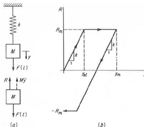
**Figure 03: Elasto-Plastic Resistance Function**
