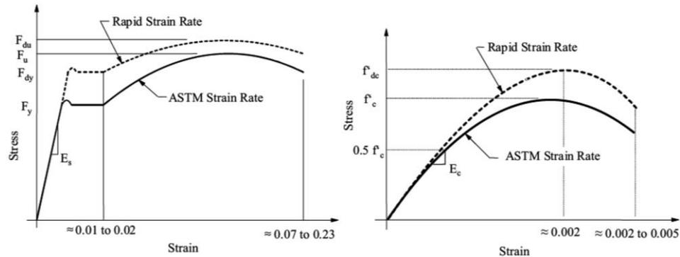
**Figure 05: Effect of Strain Rate on Stress-Strain Curve for Steel and Concrete**
