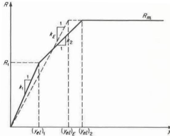
**Figure 04: Effective Bilinear Resistance Function**
