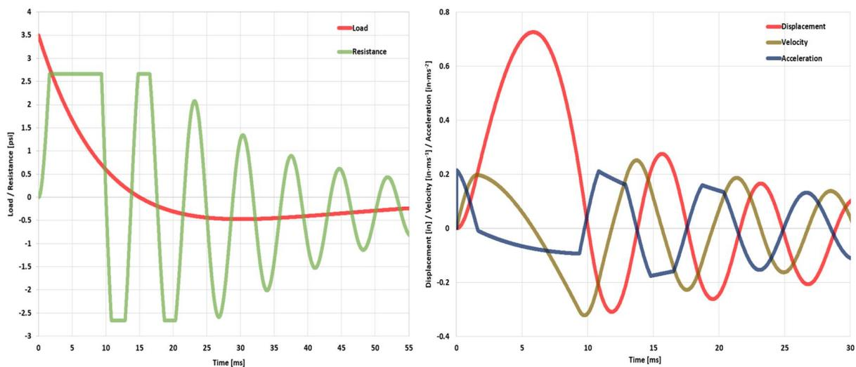
**Figure 06: Elasto-Plastic SDOF Example of Dynamic Results**
