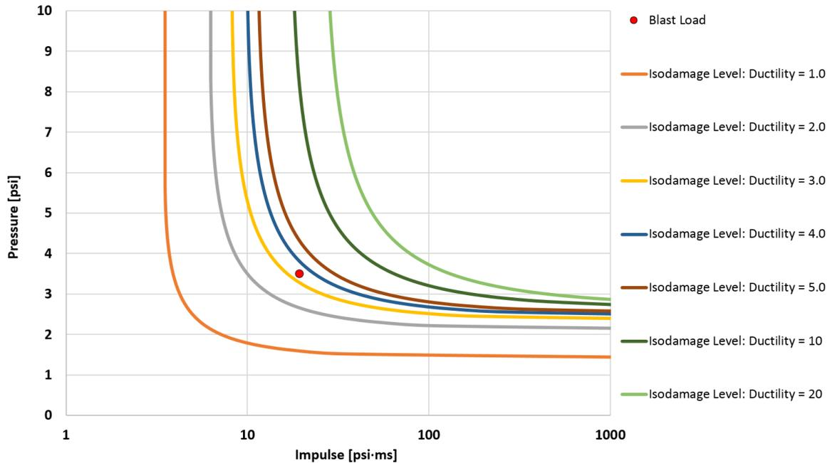
**Figure 07: Example of P-I Diagram with Several Damage Levels**
