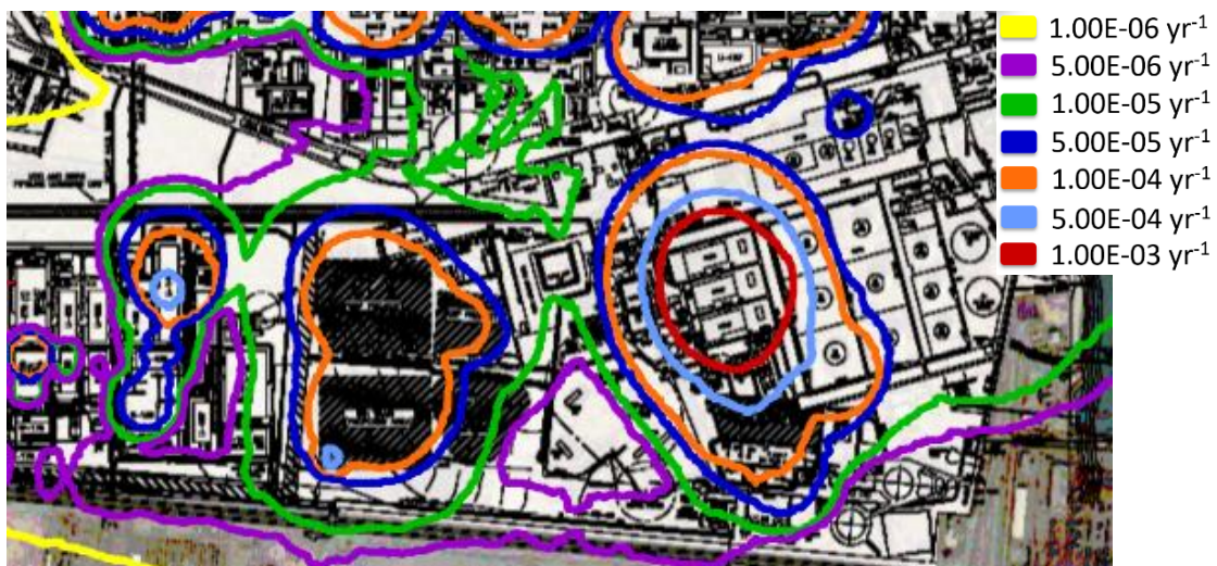
Figure 04: Example of Individual Risk Contours for a Given Process Facility
